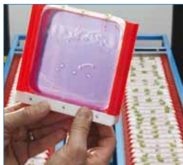
'Root Carousel': small plants are grown in Petri dishes which are moved to a camera for a quantitative assessment of root growth and structure. © Forschungszentrum Jülich
